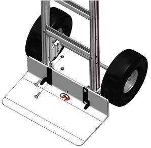
3. Attach the folding nose (A) to the inside of the brackets in the order shown: Bolt (E), flat washer (G), bracket (B), conical washer (H), folding nose (A), flat washer (G) and lock nut (F). Repeat on opposite side and tighten.
