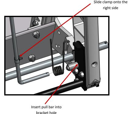
4. Take the pull bar and orient as shown. Slide clamp (F) on to the right side of the pull bar for later use. Then slide one spacer (D) and spring (E) onto the right side of the pull bar and one spacer (D) onto the left side. Compress the pull bar so the ends slide into the holes in each bracket.
