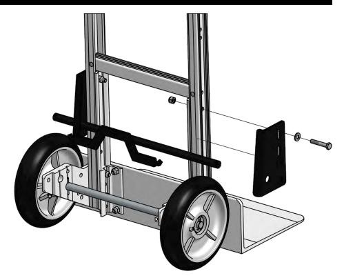
2. Attach the RH and LH brake mount plates (C, D) to the outside of the frame, mounting through the upper stiffener channel with nuts (F) and bolts (J), do not tighten completely. For 8" wheels use the upper slot in the mounting plate, for 10" wheels use the lower slot.
