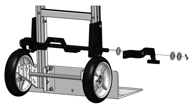
4. Slide the brake shoes apart enough to insert the pull bar (L or M) between the mounting tabs on the brake shoes. Then secure the right side of the brake axle with a cotter pin (K).
